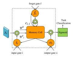
Fig. 4. An illustration of LSTM Memory Cell.
